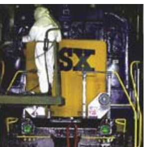
Electrostatic locomotive painting
